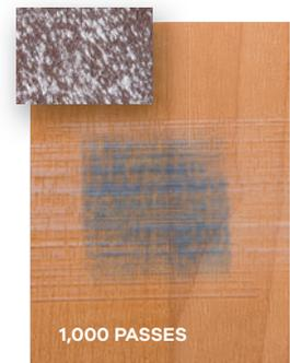
With new protective compounds from the aerospace industry and dentistry, Quantum Guard Elite's stain resistance performs over time at the same high level as the day it was installed. (Results after 1,000 passes with a sanding block, staining with a blue Sharpie and cleaning with an alcohol wipe.)
