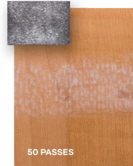
Our proprietary blend of aluminum oxide particles is suspended evenly through the urethane top coat, giving the industry's best abrasion resistance. (Results after 50 passes with sanding block.)
