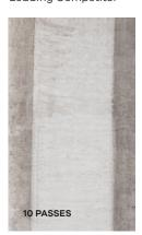
Advanced urethane chemistry and an optimized texture make resilient sheet with Quantum Guard Elite easier to clean than competitors. (Results after 10 passes with a wet microfiber mop on soiled floor.)
