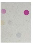
With new protective compounds from the aerospace industry and dentistry, Quantum Guard Elite leads the industry in resistance to stains, including tough medical staining agents. (Results after applying multiple medical staining agents to flooring, waiting one hour and wiping with an alcohol wipe.)
