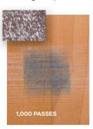
With new protective compounds from the aerospace industry and dentistry, Quantum Guard Elite's stain resistance performs over time at the same high level as the day it was installed. (Results after 1,000 passes with a sanding block, staining with a blue Sharpie and cleaning with an alcohol wipe.)
