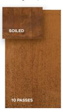
Advanced urethane chemistry and an optimized texture make resilient sheet with Quantum Guard Elite easy to clean. (Results after 10 passes with a wet microfiber mop on soiled floor.)
