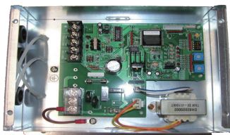
Modbus® Interface TCB-IFMB641TLE
