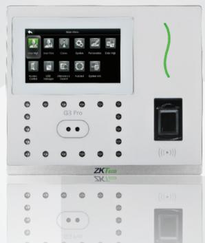
**G3** Pro is powered by Computer Vision technology like 3-in-1 contactless palm recognition, which means the terminal can perform bio-authentication with a user's palm vein, palm print, and the shape of palm at the same time once the sensor detects a hand presented.
