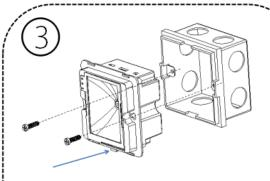
The protruded tiny area of the device pointed by the arrow as shown above should be facing the bottom. Before installing the device, connect it to the cable and test it. Then, install the device into the 86 mounting box as shown in the figure, fix the device with two M4\*15PB fasteners. Please note that the area as pointed in the figure above should be facing downwards.
