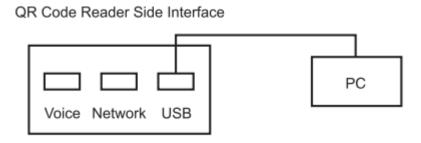
2. Then, enable "HID Keyboard" on the DEMO software setting interface, place a card or QR code (paper, electronic, mobile phone) within the reader's recognition range, the card reader will automatically obtain the information carried by the card or QR code and transmit it to the PC, which can be demonstrated by text.
