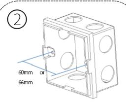
Purchase a standard 86 mounting box with an installation distance of 60mm or 66mm. Place the mounting box on the wall, mark and drill on the wall according to the box's dimensions, then fix the box with cement-bonded sand.
