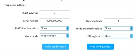
4) The user can set the parameter information of the card reader and click **Write configuration** to configure the parameter information of the QR code reader.
