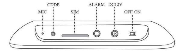
Press 【 CDDE 】 one second, alarm system is under adding remote control status.
