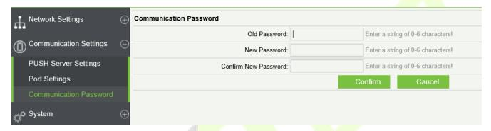
**Communication Password**: Indicates that network communication is encrypted. The default value is null, and you can set its value.
