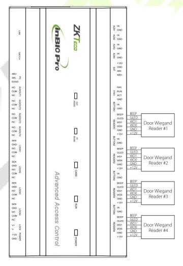
Figure 3-6 The connection between the Control Panel and Wiegand Readers
