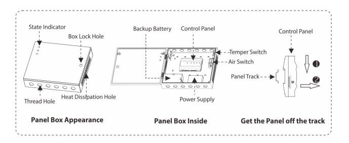
Installation steps for the control panel:
