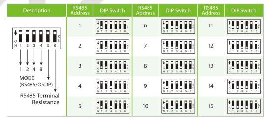
DIP Switch Setting for RS485/OSDP Communication
