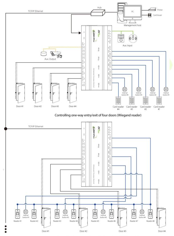
Controlling two-way entry/exit of four doors (RS485 reader)
