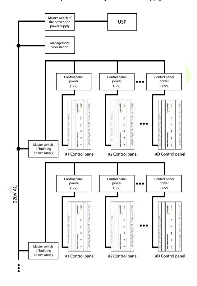
An access control operator panel is powered by +12V DC. Generally, to reduce power interference between control panels, each control operator panel should be powered separately. When high reliability is required, control panels and electronic locks should be powered respectively.
