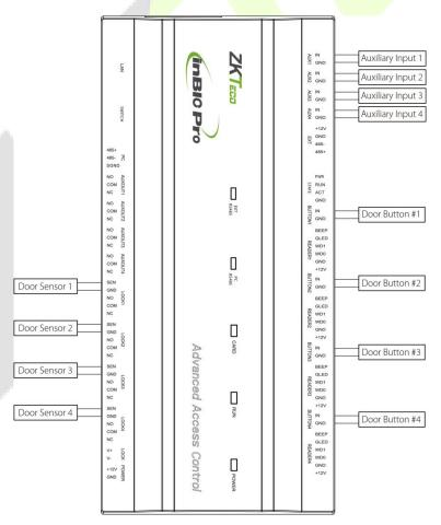
Figure 3-3 Connections between InBio460 Pro and Door Sensors, Exit Switches, and Auxiliary Input Devices
