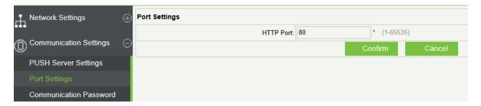
• **Http Port**: Indicates that the client initiates an HTTP request to a specified port on the server. the default HTTP Port is 80, and you can modify it according to the actual.
