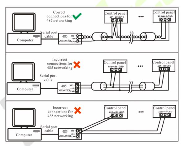
Figure 4-2 RS485 Communication System Networking
