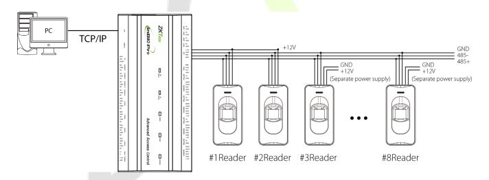
Figure 3-5 Connection between inBio460 Pro and RS485 Readers
