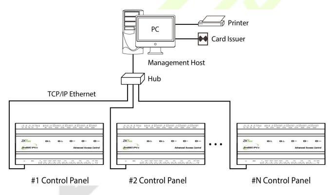
Figure 4-1 TCP/IP Communication System Networking
