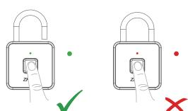
Press with one registered finger on the sensor, green LED will light if the verification is
