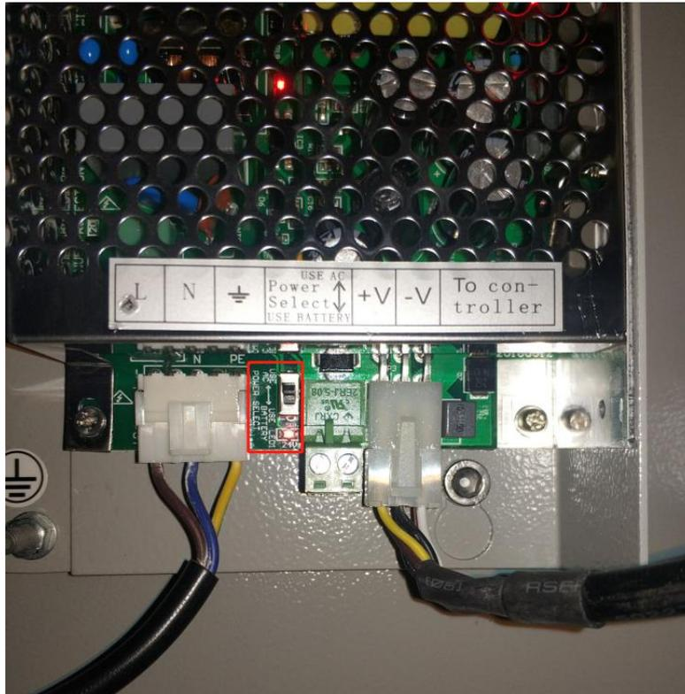
This barrier gate can be powered by 24V battery in the area without electric supply. Connection as bellows:
