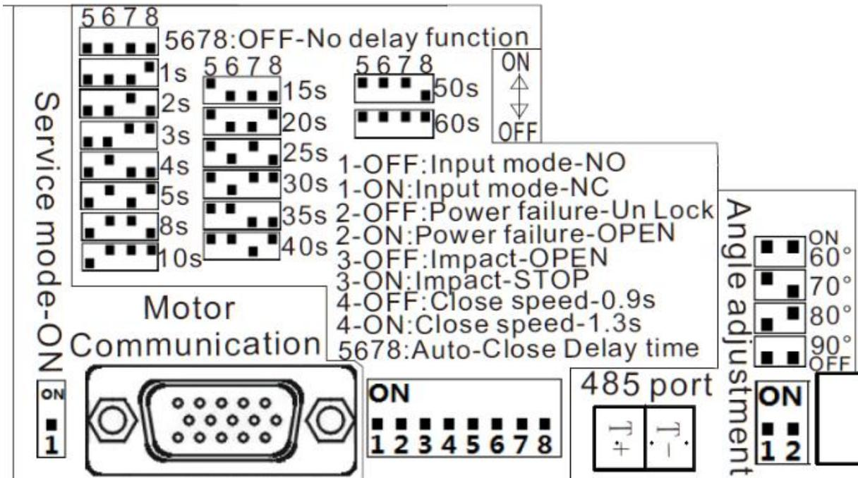
1. NO/NC mode selection, in the dip switch 1, ON for NC, OFF for NO. (Default mode, do not modify)
