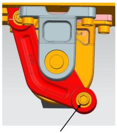
Pull boom away from dead point position (Dropping the boom)
