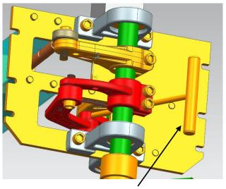
Push boom away from dead point position (Lifting the boom)
