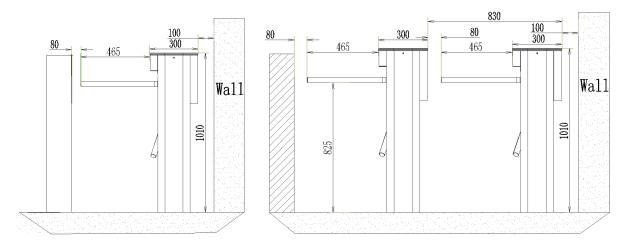
Figure 2-1 TS5000A Single channel and dual channel
