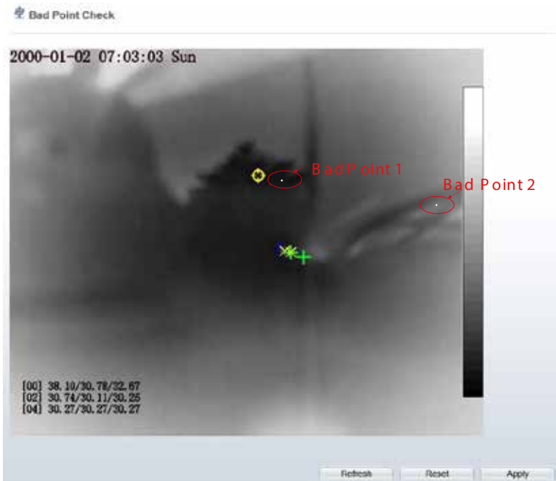
Figure 3-6 Bad point check interface
