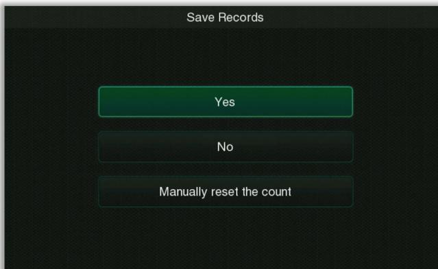
It is used to set whether to save the number of alarm records after the device is turned off, select "Yes" to save, select "No" to clear, and select "Manually reset the count" to clear count manually.
