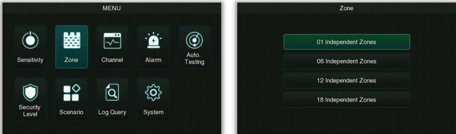
**Operation:** Press the **[OK]** button to enter the zone setting interface, then press the **[▲]/ [▼]** button to select, press **[OK]** button to save and exit.
