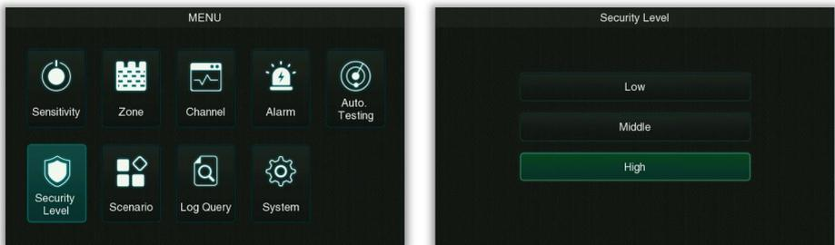
Three security levels can be set as Low, Middle and High. The higher the security level, the higher the corresponding sensitivity.
